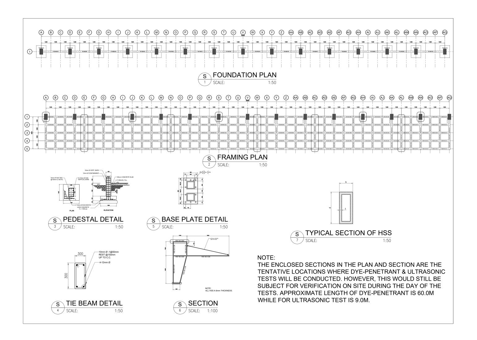
MOST CONNECTIONS BETWEEN THE BEAMS AND THE COLUMNS OF THIS TYPICAL MEMBER WILL BE TESTED WITH DYE PENETRANT TEST. THE TEST WOULD FOCUS ON THE BEARING PLATE AND THE OTHER BUILT-UP SECTION CONNECTIONS. THE LINEAL METER FOR THIS DYE-PENETRANT TEST IS APPROXIMATELY 60M WHICH SHALL BE SELECTED RANDOMLY. THERE WOULD BE AT MOST THREE (3) ULTRASONIC
